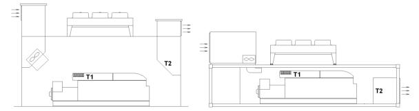
The minimum recommended air change ratio (C) must be observed to maintain the required air quality and prevent unwanted gas accumulations (refer to Section  $\Rightarrow$  Potentially explosive Atmospheres as per TA1100-0110). The calculation is based on TA 1100-0110 and is C<sub>min</sub>= 50h<sup>-1</sup> for JENBACHER modules.
